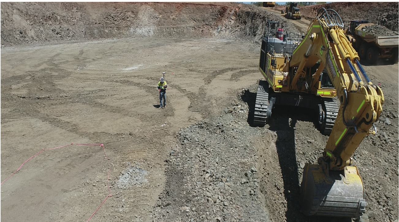
Image 9 – Digger operator waiting for the grade control geologist to mark up ore body (outlined in red rope at bottom left of image)
