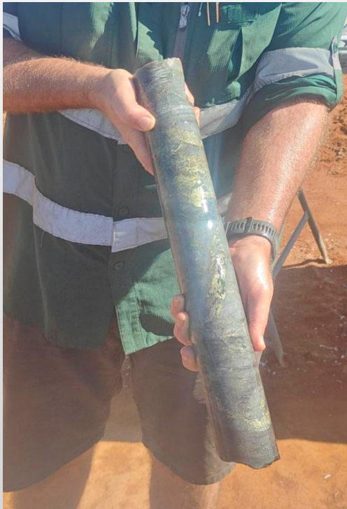
BHRCD029 core from 339.9m to 340.45 m showing chalcopyrite hosted in quartz veining
