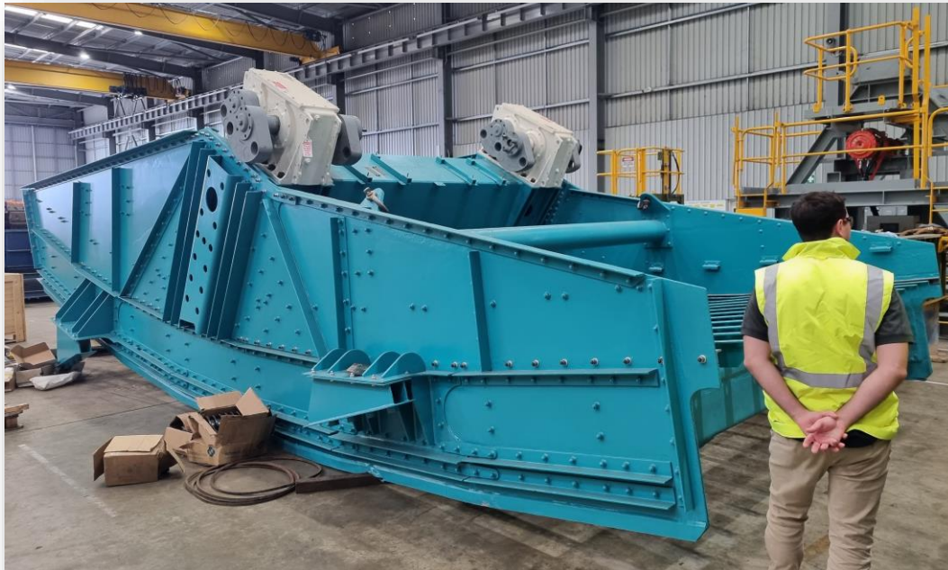
Figure 3: Refurbished Schenck banana screen
