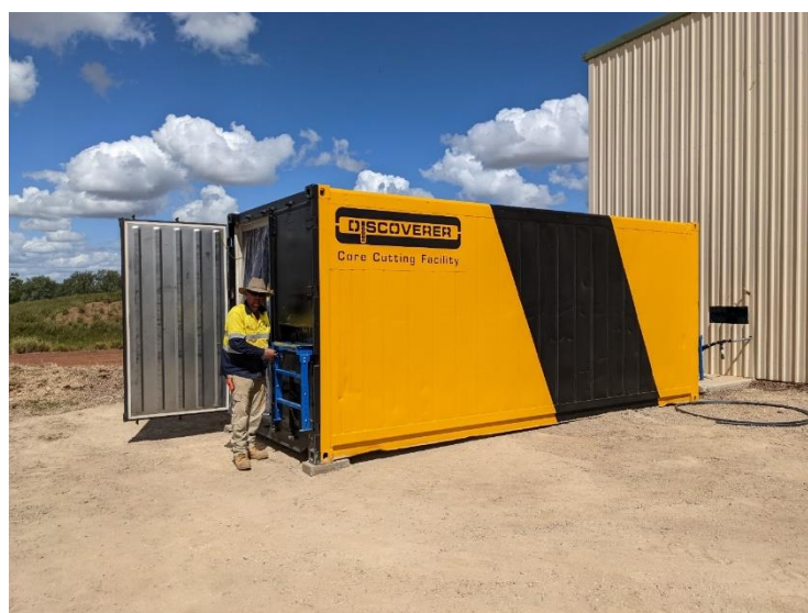
Figure 21: Purpose-built core cutting facility incorporating machine guarding, dust management and air conditioning
