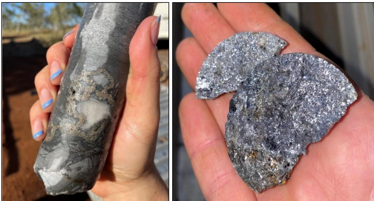
Figure 1 - (left) Buff-coloured colloform sphaerite replacing carbonates in pseudo-breccia (JB22_02) and (right) near-complete replacement of carbonates by galena (with minor sphaerite) in JB22_02.
