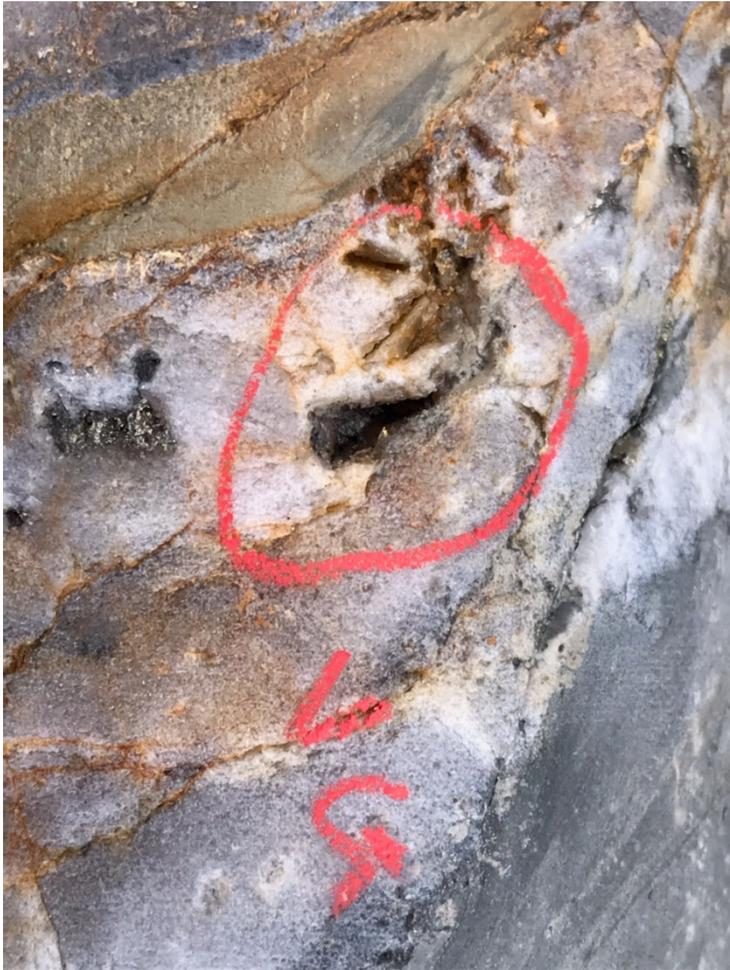
**Figure 5 Further Visible gold within the quartz vug**
