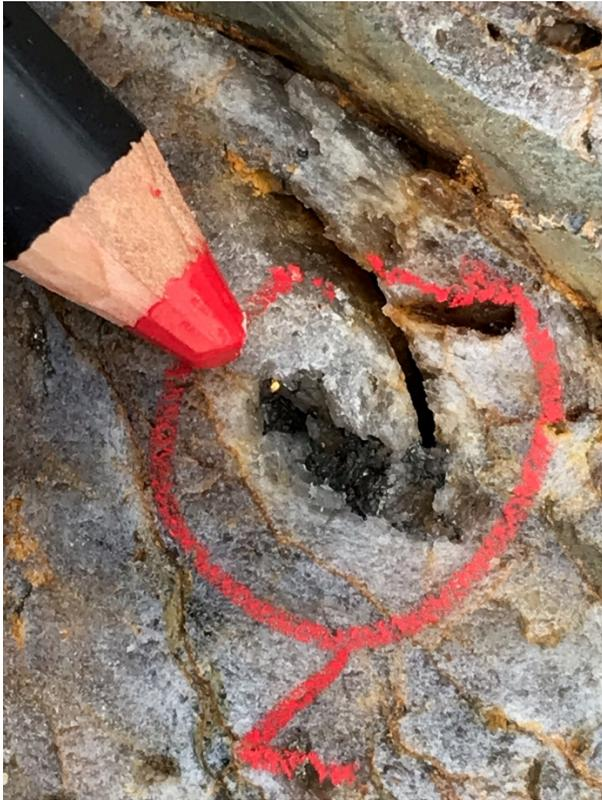
**Figure 3 Visible gold in quartz vug**
