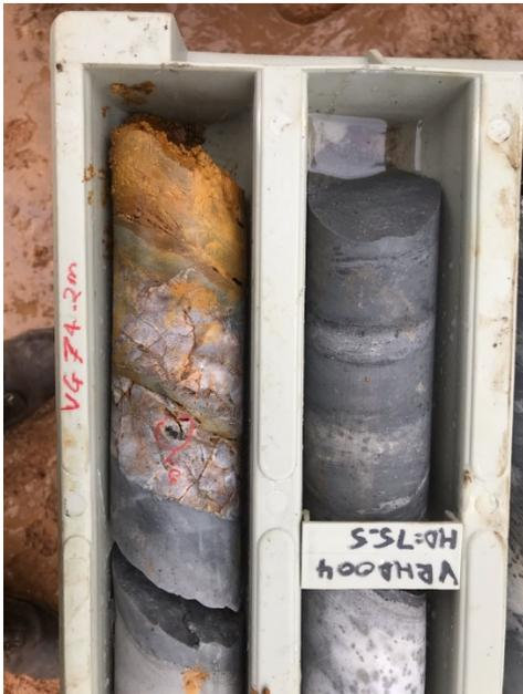
**Figure 4 Visible Gold shown in the red circle in the HQ core.**
