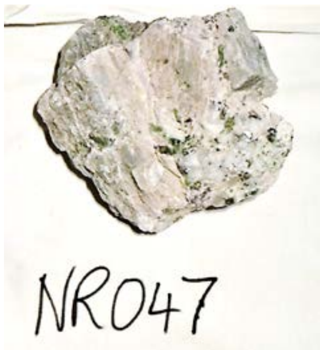
Figure 6: Albite-spodumene-quartz-tourmaline rock. About 15% spodumene
