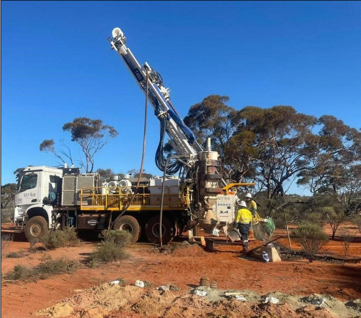
**Figure 9.** AC drilling at Emu Lake – September 2021
