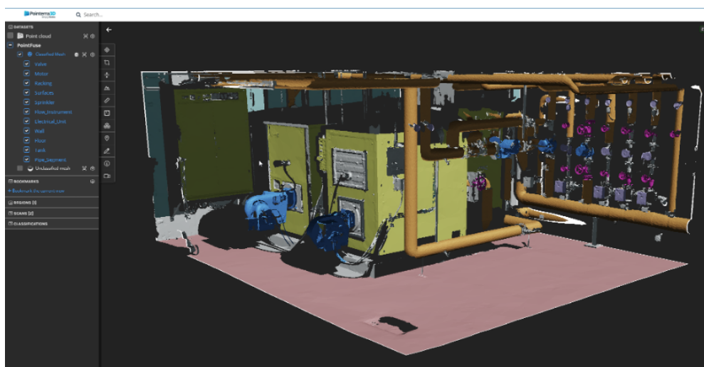
Pointfuse classified mesh created from point cloud
