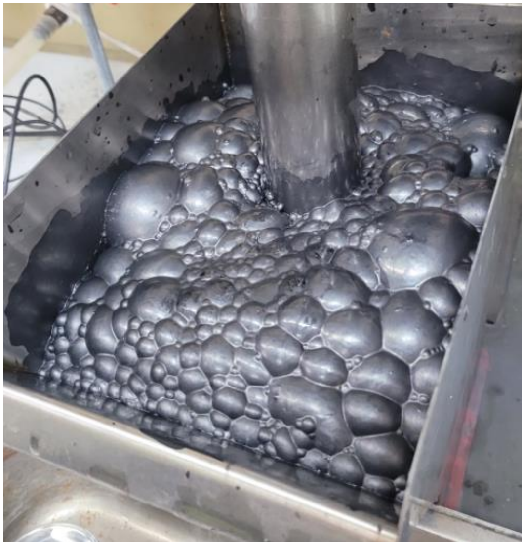
Figure 4 – Flotation test on Sarytogan graphite at the IMO Metallurgy laboratory, Perth
