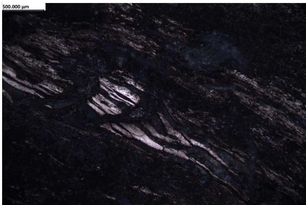
Figure 6 - Thin section photomicrograph of St-47-56.4 (21_1310_209) in reflected light (XPL, 5x objective). Thick graphitic ribbons in graphite schist with late-stage quartz veins crosscutting the fabric.
