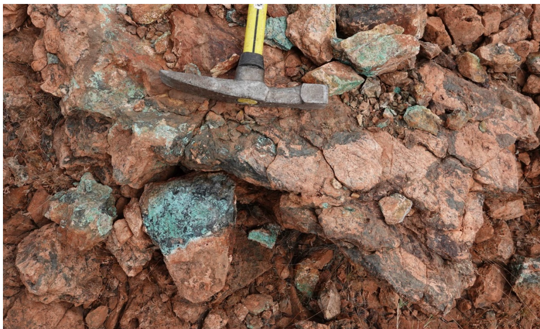
Figure 20. Breccia with coarse albite actinolite magnetite infill and abundant malachite on fractures.
