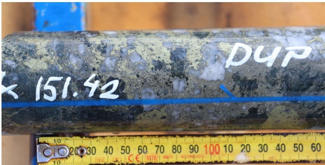
Figure 16. HMTRDD001 151.5m Chalcopyrite-Pyrrhotite as matrix infill in a quartz vein breccia. Main Trafalgar lode. The interval 151.42-152.55 assayed 0.5g/t Au and 7.65% Cu.
