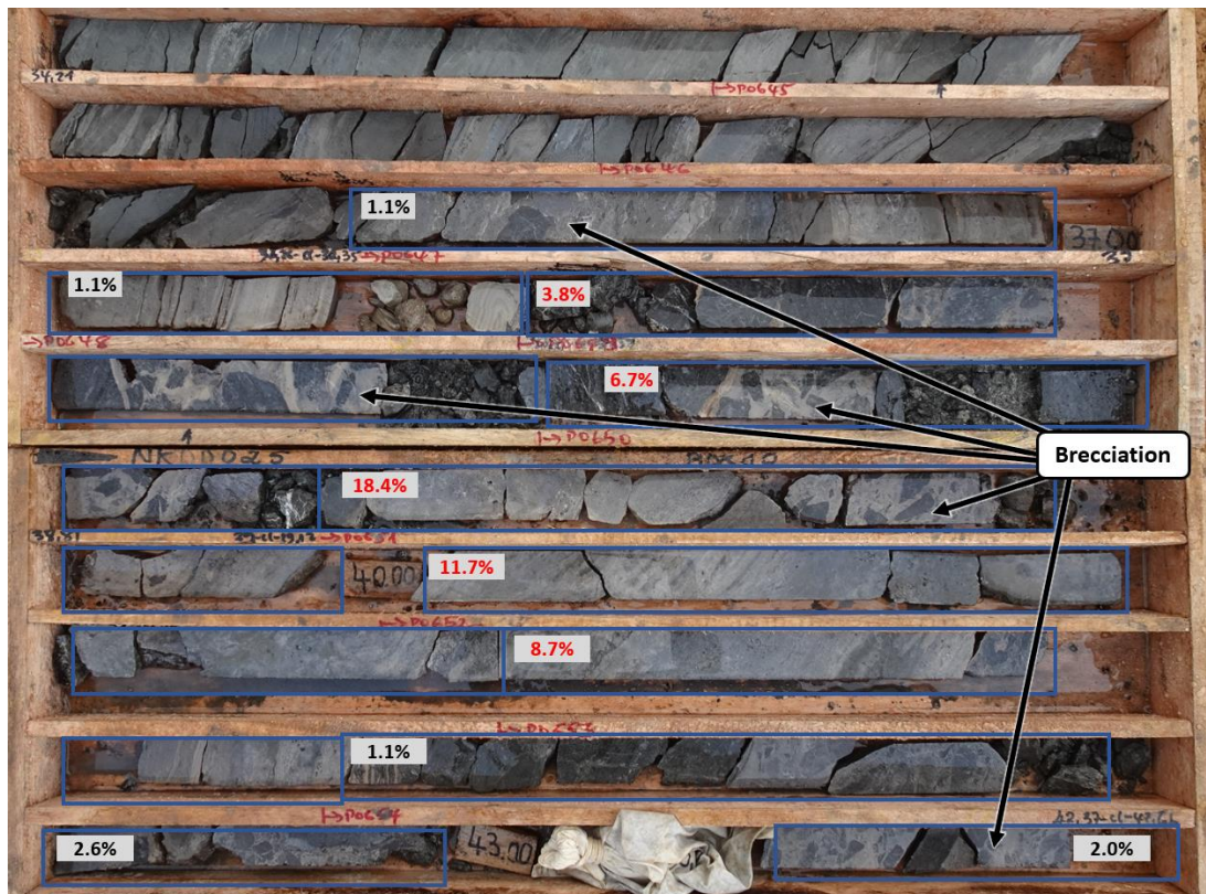
Figure 4 – NKDD025 – Displaying Zn+Pb% grade in core and region of breccia-related mineralisation (36.3m to 45m).
