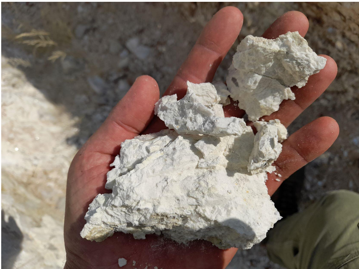
Figure 1: Example of unaltered spodumene identified at surface at the large mine working on EPL 7345 (Uis Lithium-Tantalum-Tin Project) - Note: Visual estimates should not be considered a proxy or substitute for laboratory analysis. Assay results are expected to be received in late November 2022, subject to turnaround times at the laboratory. Sample Tag: U4674; Sample location – E: 472460 and N: 7639905
