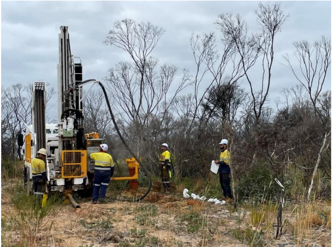
Photograph 1: Aircore drilling at the Mount Ridley Project.
