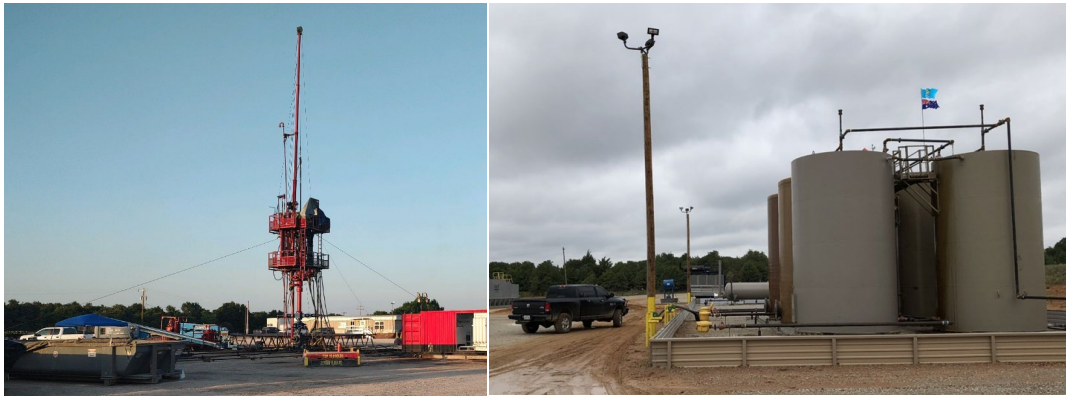
Figure 5. Snubbing unit (left) and production facilities (right) on location at the Flames Well, Carter County, Oklahoma
