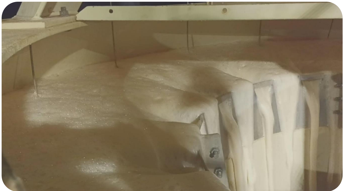
Trial radial froth launder operation in flotation cell 1 on 28 October 2022
