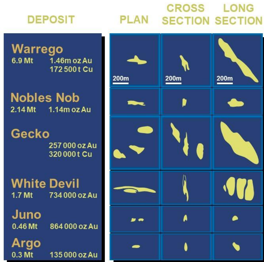
Figure 5: Geometries of Major Tennant Creek Orebodies, noting the typical constrained plan/horizontal footprint.
