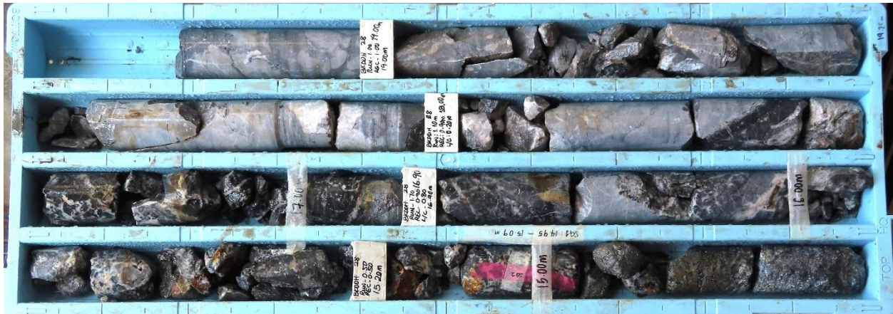
Figure 7: Section BKDDH-28, illustrating the intensely hydrothermally alteration across the shallow Pedawan and Bau Limestone formations.
