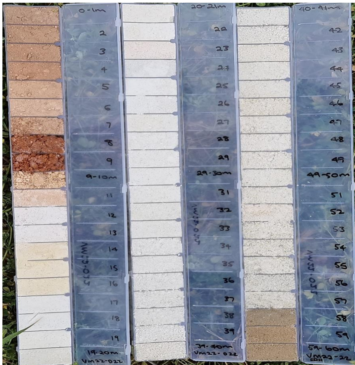
Figure 2 Chip tray samples for drillhole VM22-022 within EL6733. Total depth was 60 metres. Each rectangle contains representative material for each one metre in depth.
