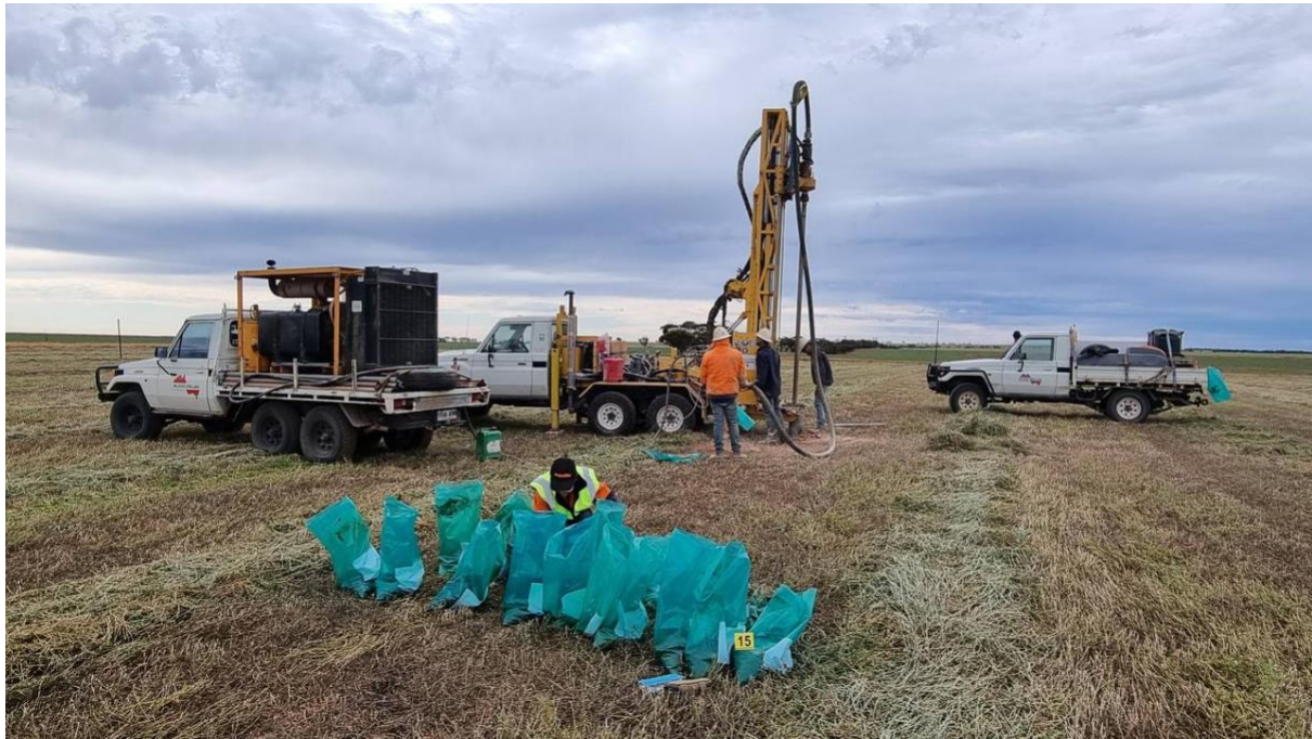
Figure 1: Aircore drilling hole VM22-015 at the Poochera Project
