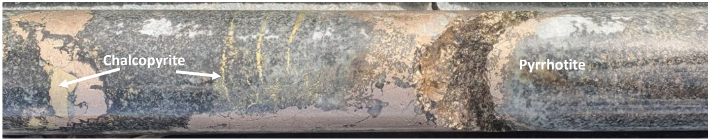
Figure 5. Massive sulphides in TMDD0001, chalcopyrite, pyrrhotite and pyrite observed, 841m depth.
