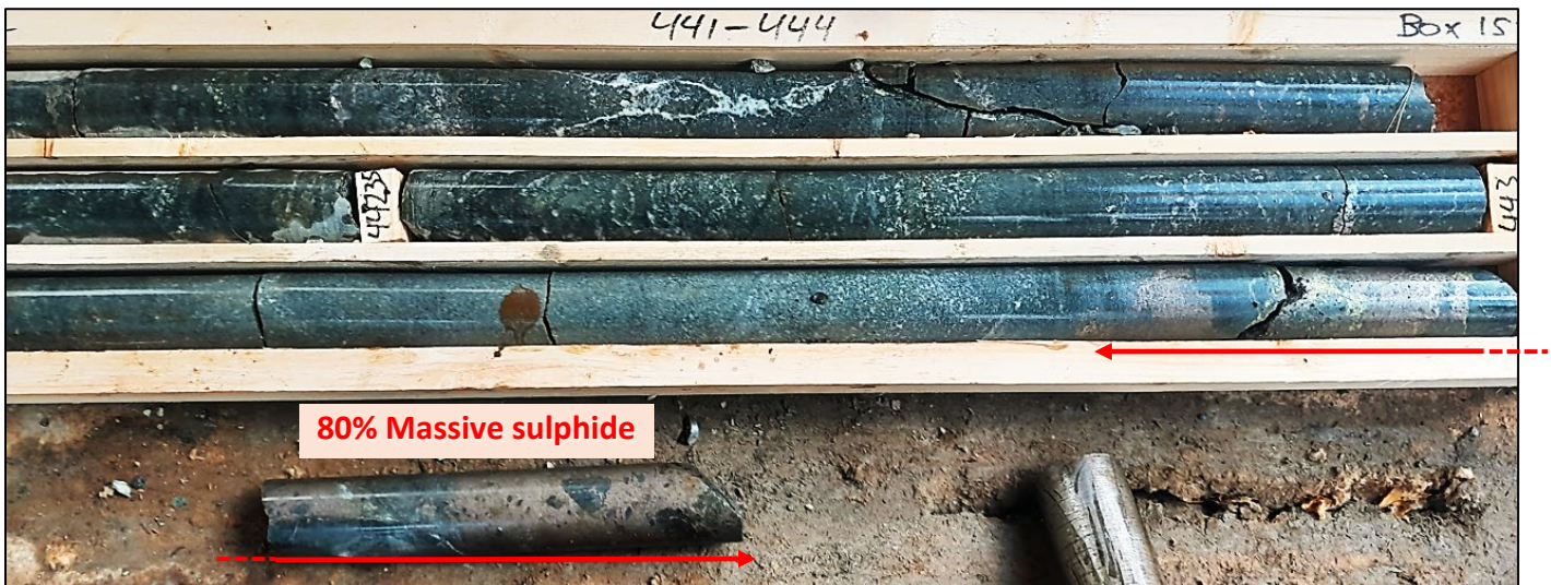
Figure 4: Basal Massive Sulphide zone comprising pyrrhotite, chalcopyrite and pentlandite (443.7m-444.25m highlighted)
