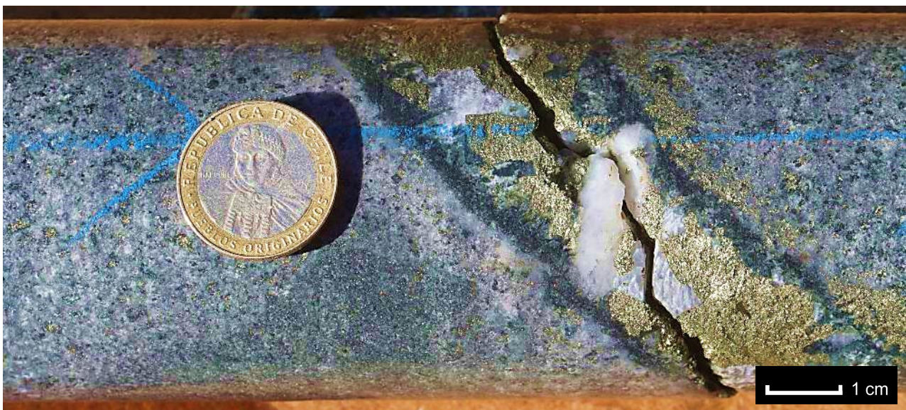
Figure 4: Vein hosted chalcopyrite mineralisation logged in CMLCD010.
