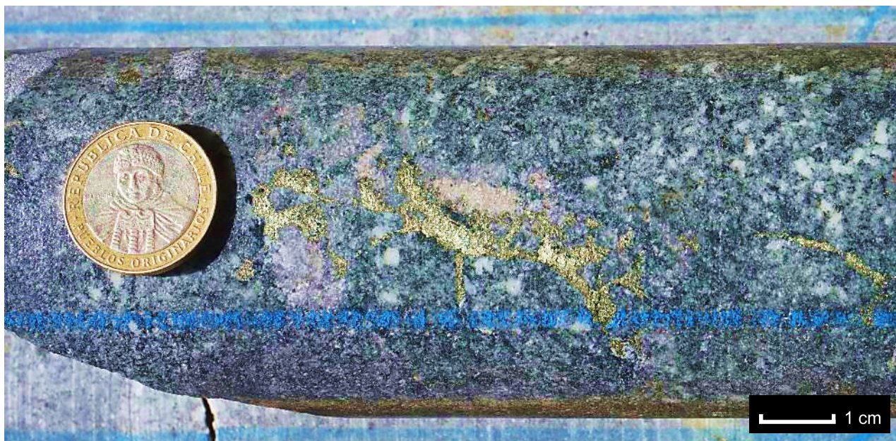
Figure 1: Core from CMLCD010 with visible copper sulphides 6 , refer Appendix E
