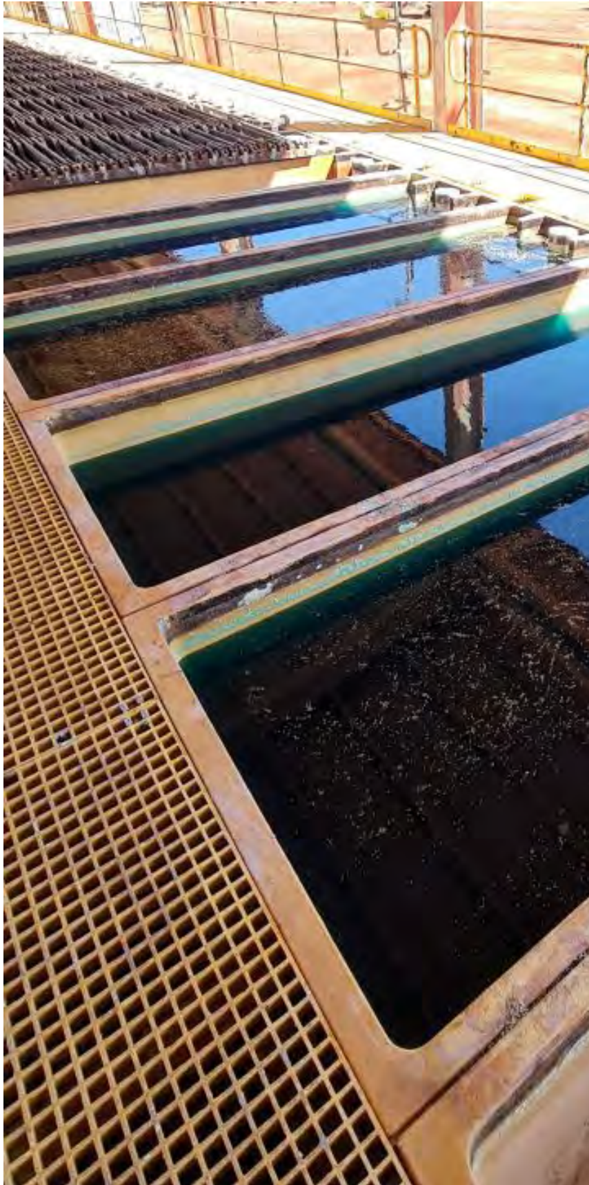
Image 7 / Hydro testing EW cells following removal of cathodes and anodes and clean up
