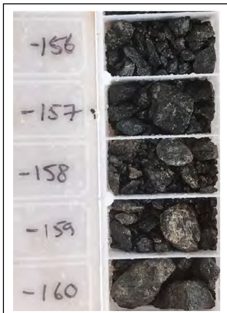
Image 13 / RC drill chips: 22SKRC001 146m to 165m, Gabbro with stringer pyrrhotite/pyrite/chalcopyrite. 19m at 5,000 ppm Cu, 1,297 ppm Ni, 100 ppm Co, 0.28 ppm Pd, 0.11 ppm Pt
