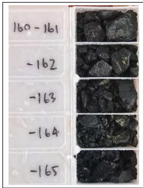
Image 13 / RC drill chips: 22SKRC001 146m to 165m, Gabbro with stringer pyrrhotite/pyrite/chalcopyrite. 19m at 5,000 ppm Cu, 1,297 ppm Ni, 100 ppm Co, 0.28 ppm Pd, 0.11 ppm Pt
