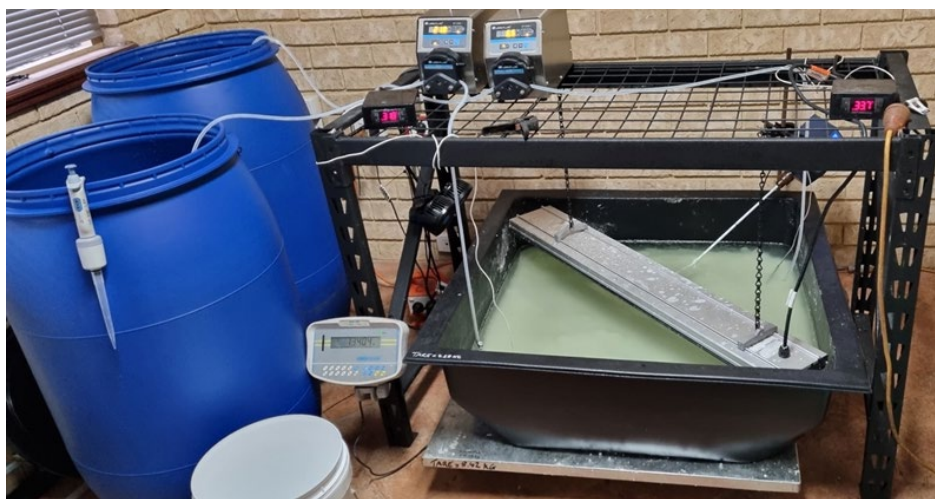
Figure 7: Leonite precipitation set-up
