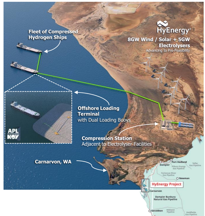
Figure 4: Overview of the HyEnergy Project to evaluate export using a compressed hydrogen supply chain
