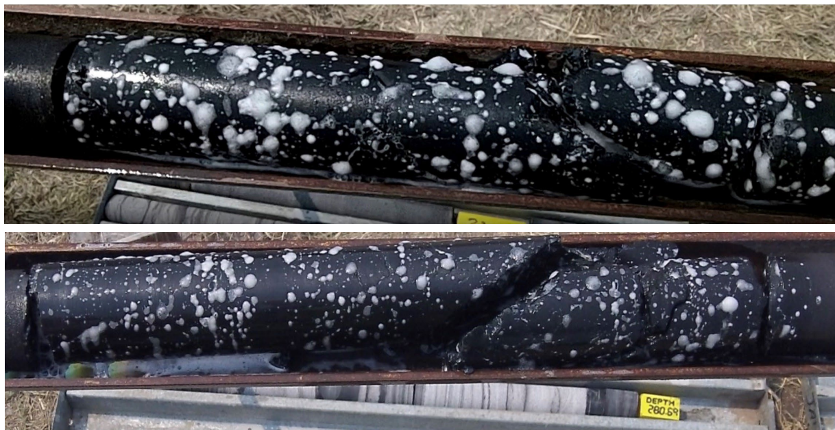
Figure 2: Core well 271-23C visible gas emissions observed from core samples at depths between 230-280m
