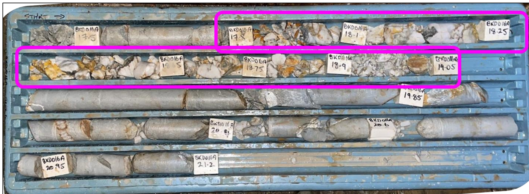
Figure 5: Recovered drill core from BKD016A, showing the quartz reef of interest between 17.80 and 19.05m
