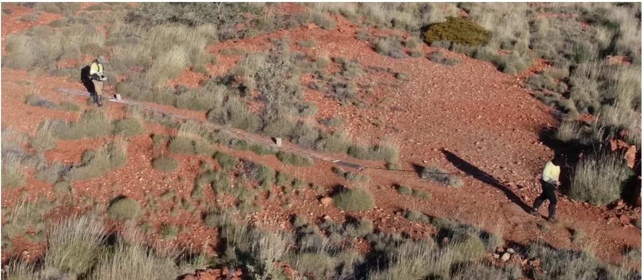
Photo 1: Drone view of the DGPR data acquisition process at Tambourah - a very low impact exploration method.
