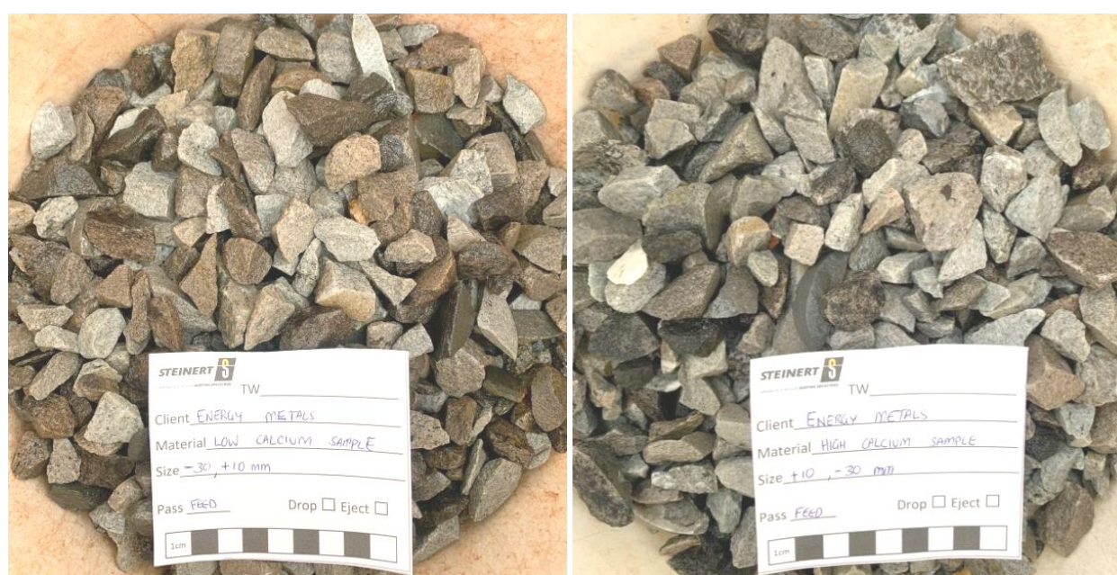
Figure 4 – Low-carbonate (left) and high-carbonate (right), +10mm feed samples for ore sorting.
