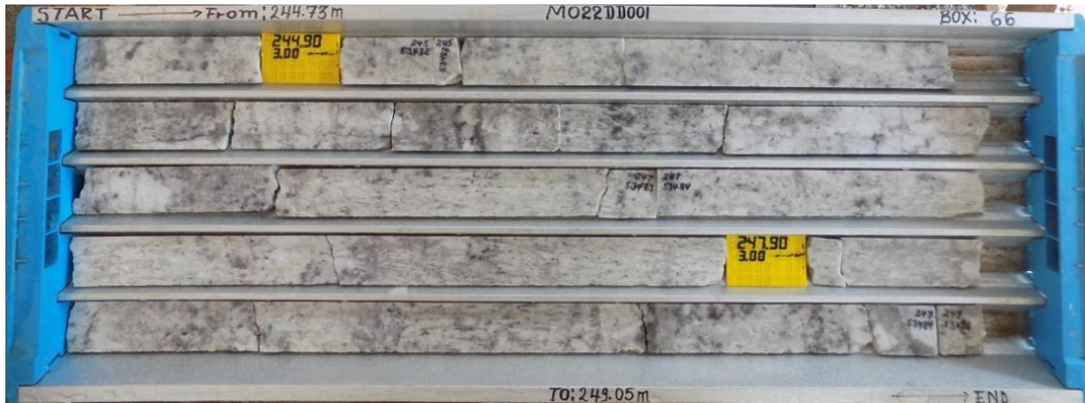
Figure 1: MO22DD001 245-249 4m@2.47% Li 2 O showing coarse spodumene crystals
