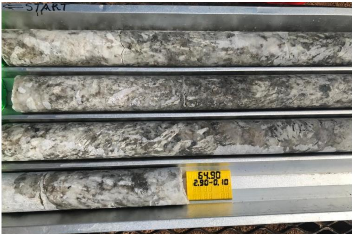
Figure 2: Close up visible spodumene from MO22DD001 at 64.9m downhole
