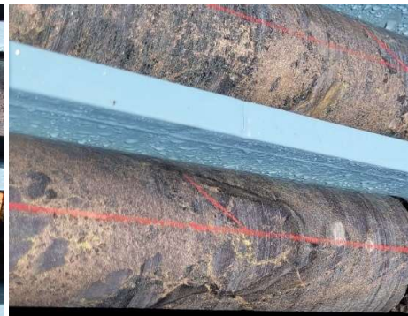
Photo 2: Matrix breccia sulphides, 351m.
