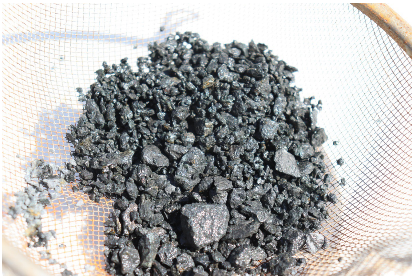
EDRC22126: Up to 5% disseminated nickel and copper sulphides visually logged from 98 m downhole. 1 m @ 4.6g/t (3E), nickel, copper and rhodium and iridium assays pending. Within broader 9 m @ 2.31 g/t (3E).
