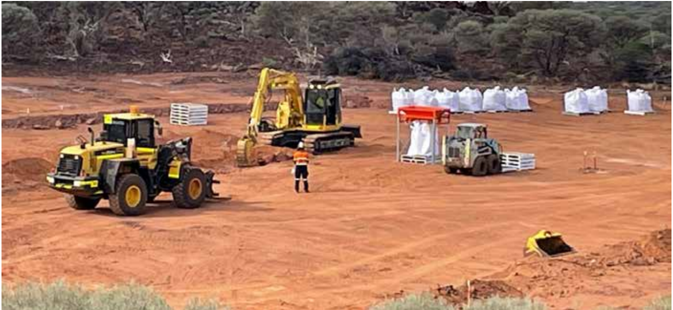
Figure 6 – Costeaming operations to extract, sample and bag mineralisation at Barrambie. Source: Neometals.
