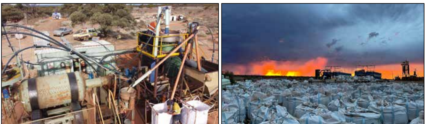
Figure 7 – Milling and gravity beneficiation of mineralisation to produce 130t MGC bulk sample. Source: Neometals.
