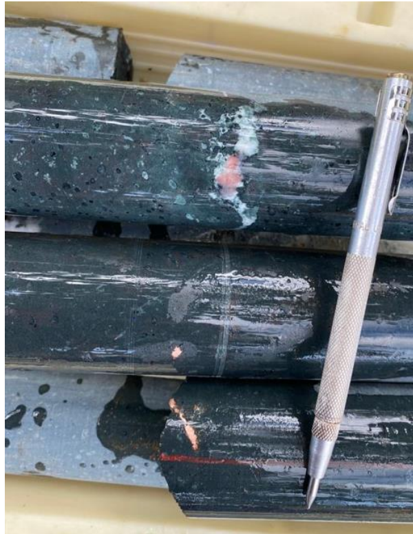
Figure 1B: 22RRD-001 Altered magnetic basalt with native copper slugs at 126-127m depth.
