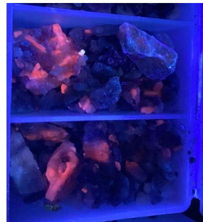
Image 2: TMBRC003 from 18.0m to 20.0m under UV light showing spodumene in pink
