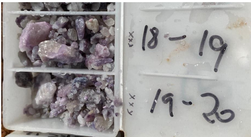
Image 1: TMBRC003 from 18.0m to 20.0m interval within 13.0m pegmatite intercept in natural light showing lepidolite and spodumene mineralisation
