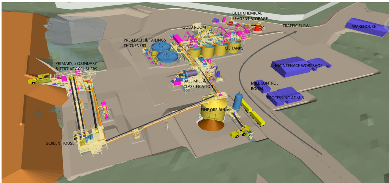
Figure 2: Isometric design of the Bellevue Gold Processing facility (looking East)
