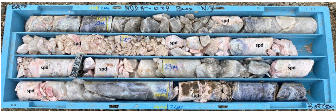
Figure 11: NDDH004 Core-tray #7. Spodumene labelled spd. Pale blue = albite (variety cleavelandite), purple = lepidolite, grey = quartz
