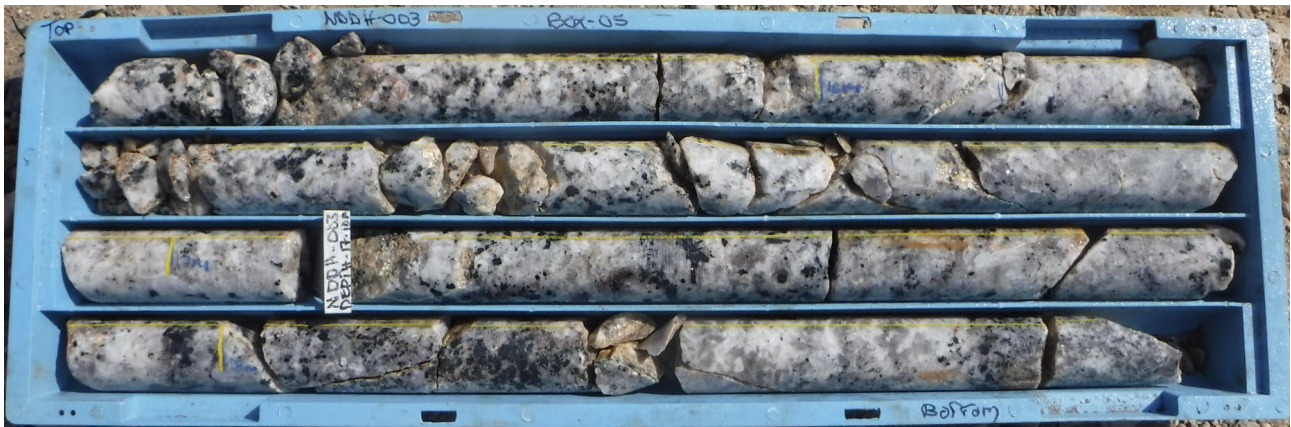
Figure 6: Example of the typical wall-zone pegmatite intersected in NDDH003.
