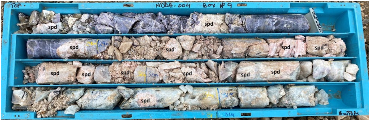
Figure 12: NDDH004 Core-tray #9. Spodumene labelled spd. Pale blue = albite (variety cleavelandite), purple = lepidolite, grey = quartz
