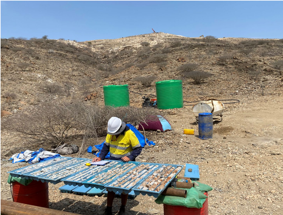
Figure 2: Core-trays laid-out on makeshift core rack at site. Note drill-rig in background on top of hill, set-up on drill-hole NDDH004. Geologist Neil Scholtz logging drill-core from NDDH004.
