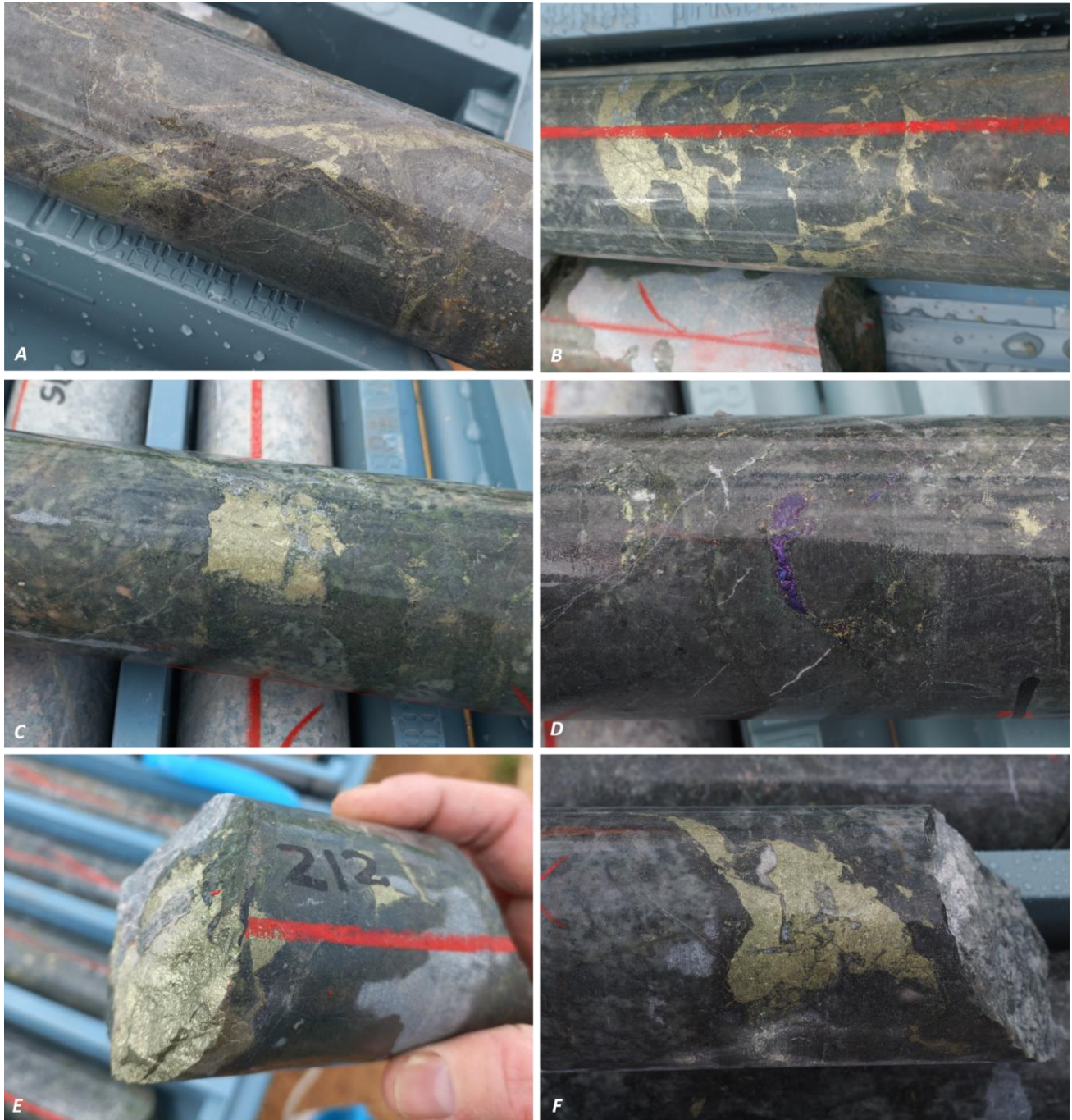
Figure 2. Various styles of copper mineralisation from the upper portion of hole 22MYDD417 (HQ drill core - 63.5mm diameter), which returned 117.0 metres at 0.55% Cu, 0.12g/t Au & 33ppm Mo from 134.4m. A) brecciated andesite displaying well developed chalcopyrite/pyrite infill associated chlorite and sericite alteration from 151m; B) polymict andesite/diorite breccia with strong chalcopyrite (yellow) infill from 173m; C) brecciated diorite with strong chlorite alteration hosting a large patch of chalcopyrite with minor carbonate from 191.1m; D) strongly fractured and chlorite-altered andesite with an elongate patch of bornite (purple, centre) and minor chalcopyrite (yellow) from 206.9m; E) chlorite-altered andesite breccia with strongly developed chalcopyrite from 212m; F) large patch of chalcopyrite (yellow) surrounded by magnetite (black) within a brecciated and strongly altered diorite host from 221.3m.
