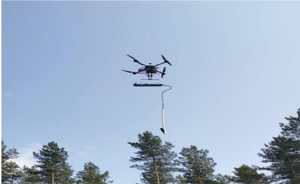
Figure 3: Image of Drone MAG system
