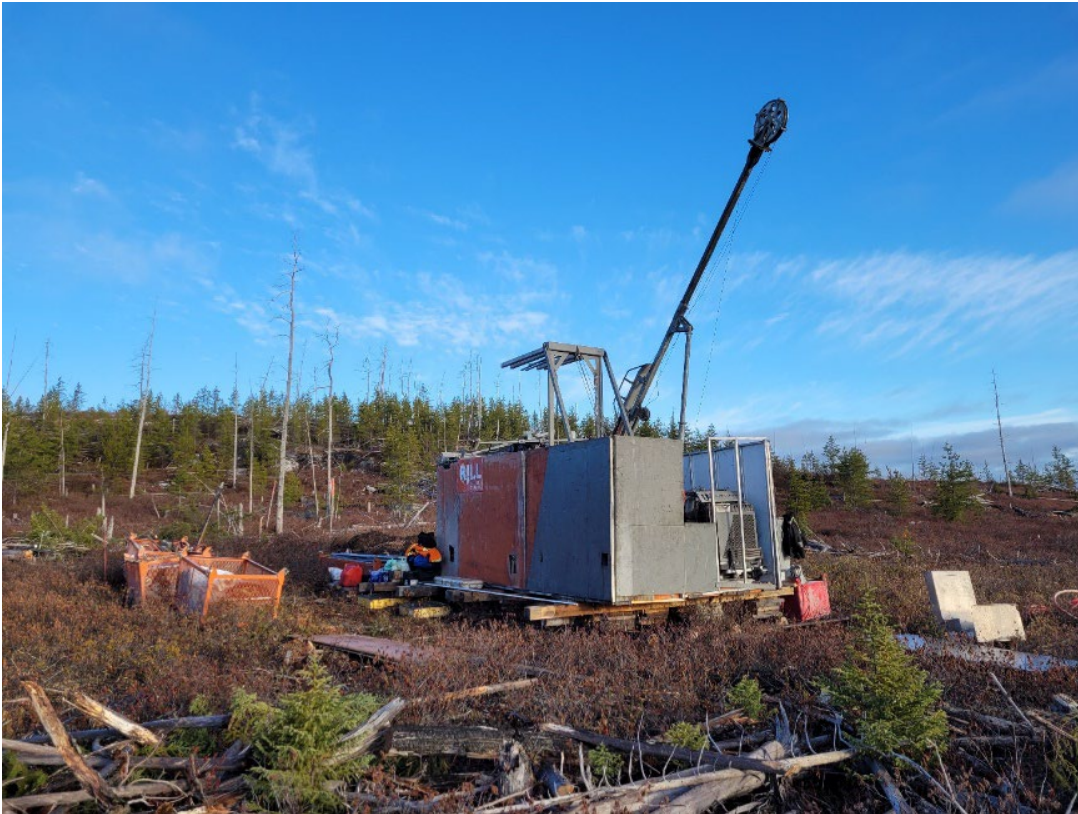
Figure 2: Diamond drill in place and drilling the maiden drillhole for Cygnus at Pontax Central. Targeting down dip of known high grade mineralisation.
