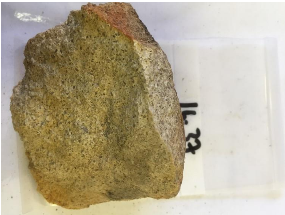
Figure 6 – Rock chip of outcropping from Figure 5 silicified caprock of fine brecciated quartz in a clay matrix
