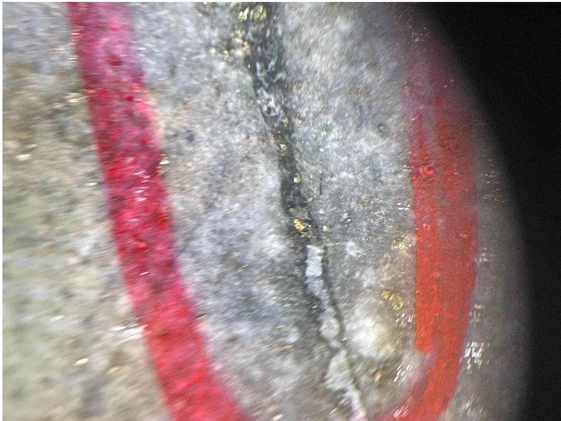
Figure 8: TUDDH 608. Visible gold at 602.6-603.0m within mm-scale vein. Grade: 80.02 g/t Au
