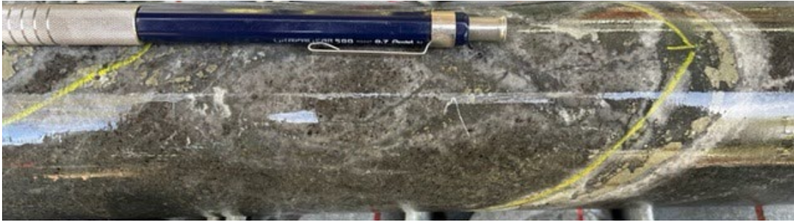
Figure 6: TUDDH 608. Gold-bearing veins at 600.5m. Grade: 21.69 g/t Au
