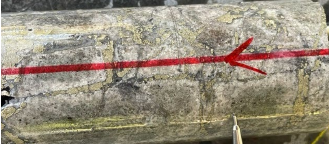
Figure 9: TUDDH 608. High-grade material hosted within mm-scale ladder vein at 606.5m. Grade: 54.54 g/t Au
