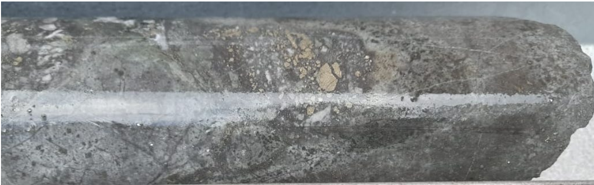
Figure 4: TUDDH 608. Mineralized Andesite core at 596.7-597.9m. Grade: 85.41 g/t Au over 1.2m
