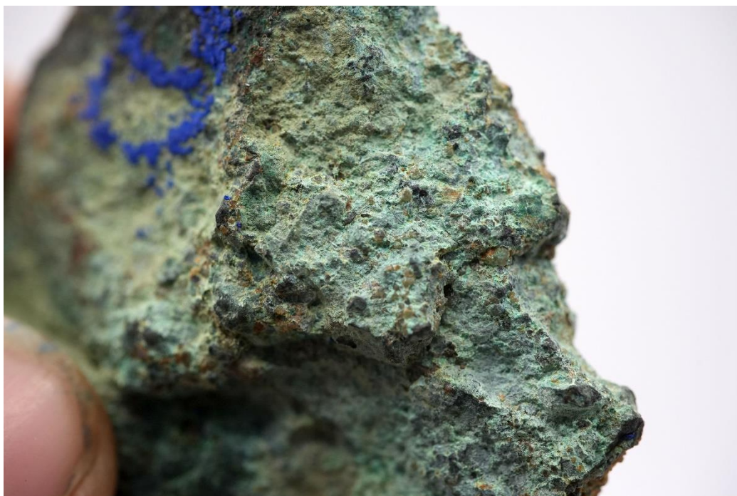
Figure 1: Copper oxide coated chalcocite in sandstone from the Discovery Zone sample A1199b. This sample comes from 81° 57' 18.58", -26° 12' 0.86".
