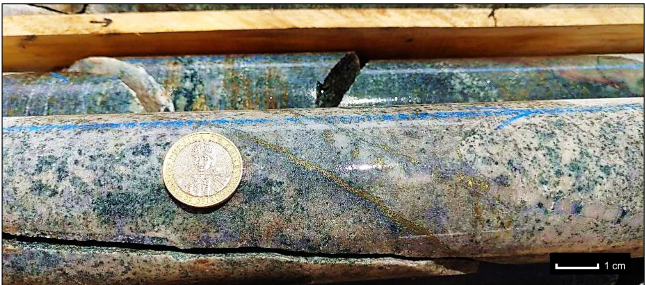
Figure 4: Chalcopyrite and Molybdenum mineralisation logged in CMLCD011 (347m) associated with phyllic alteration (Refer Appendix E).
