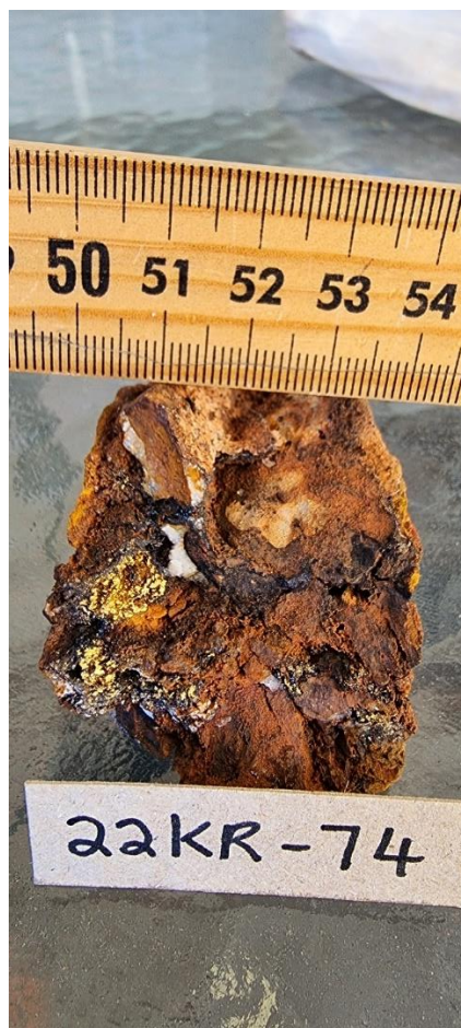
Figure 5: 22KR 74 – roddeledongate vein exposed at 0.90m below surface possibly pitching southeast (C3)
