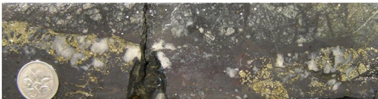
Figure 53: Mineralised magnetite-chalcopyrite-pyrite breccia in felsic metavolcanic (DCDH01: 331.8 m) (Minotaur Exploration Limited, 2020).
