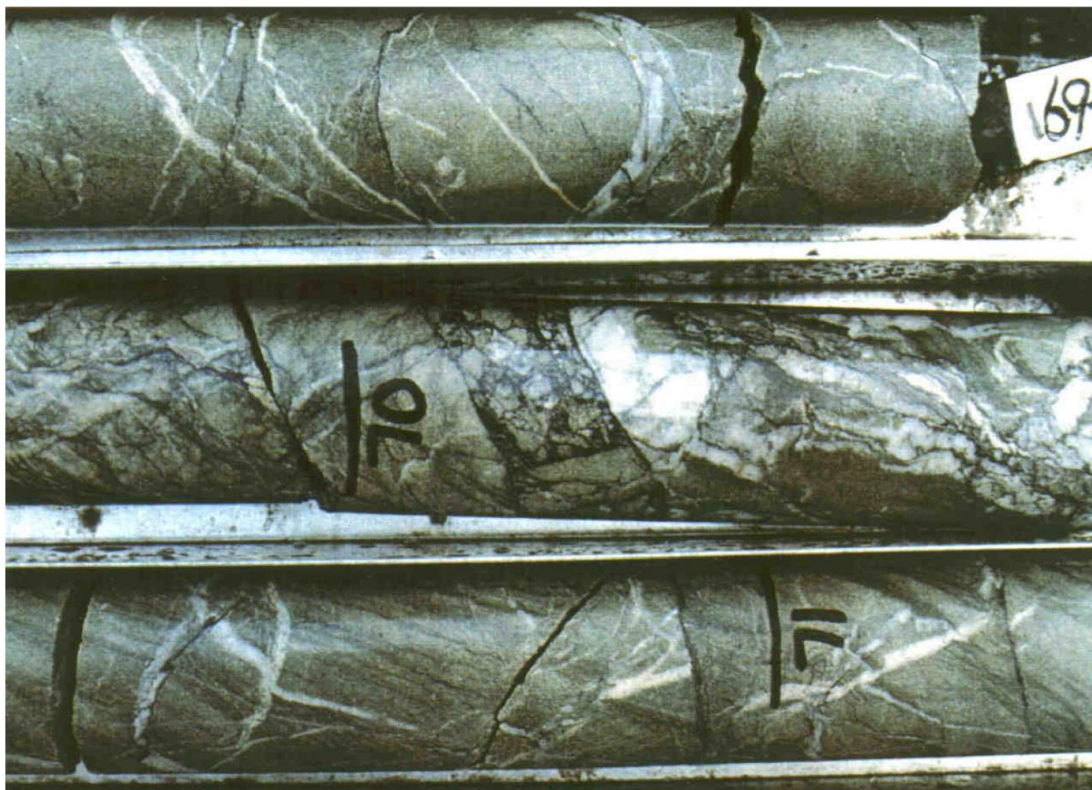
Figure 39: Photograph of drill core from MDD-001 (Gettysberg prospect). Typical chalcedony-comb quartz vein stockwork mineralised zones in sericite-altered, thinly bedded sandstone. Assay 70–71 m @ 0.37 g/t Au (Borthwick, 2017).
