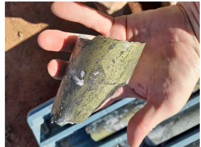
Figure: KSNDH015 - 71.9m: Chalcopyrite vein. Sample interval 71.6m to 72.3m: 5.5% Cu, 0.5g/t Au, 13g/t Ag.
