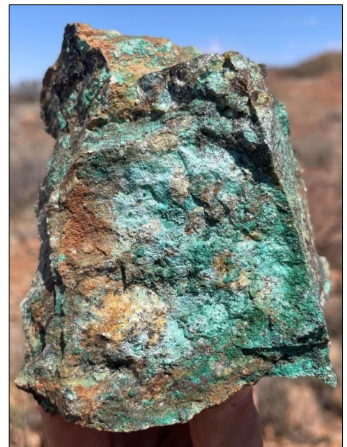
Figure 1: An example of supergene-enriched malachite mineralisation from skarn-like Cu lodes at the Bonya West prospect (sample JE0171).
