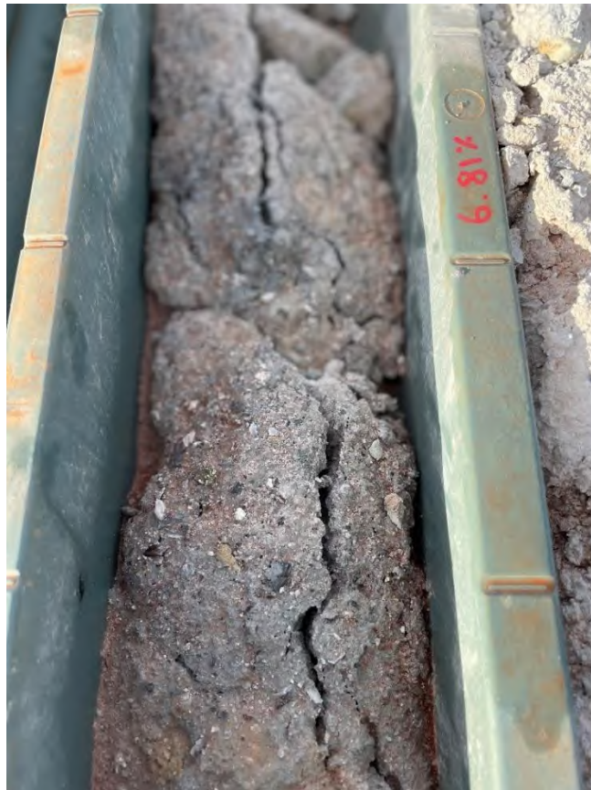
Figure 3: Example of excellent sample recovery from sonic drillhole EHS01 through relatively unconsolidated and hard and soft Navajoh unconformity hosted transitional mineralisation.
