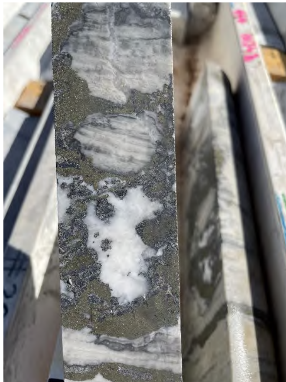
Figure 5: Fresh Sulphide Mineralisation (pyrite, sphalerite galena) crosscutting and replacing siliceous dolomite EHD027
