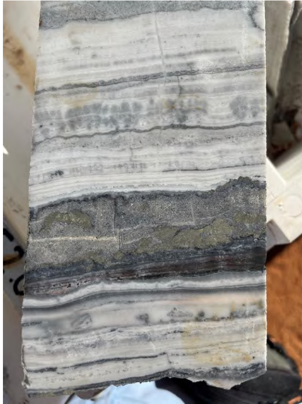
Figure 4: Fresh rock MVT style replacement mineralisation in diamond hole EHD027 Tonka Prospect
