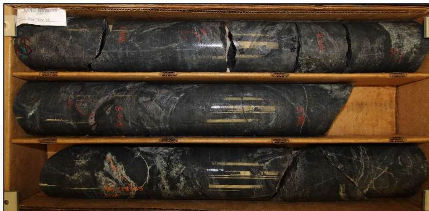
Photo 1 – Large diameter core from hole WT-22-160, showing section 25m at 2.06% Cu and 0.61g/t Au.
